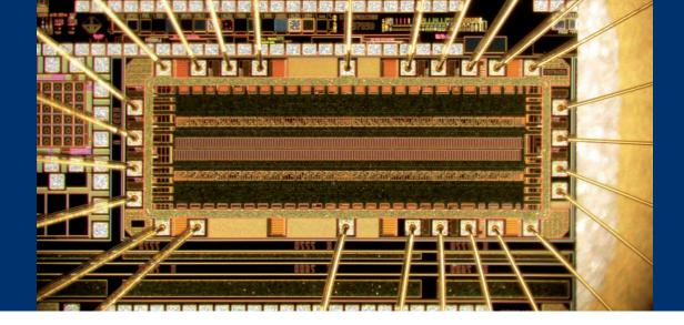
Integration of tailored CMOS readout electronics on the same chip allows adaptation of the sensor performance according to the requirements of the intended applications. The SPADs can be used as 1D or 2D arrays and, by integration of quenching resistors on the pixel level, even as silicon photomultipliers (SiPM).
